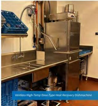
Ventless High-Temp Door-Type Heat Recovery Dishmachine
