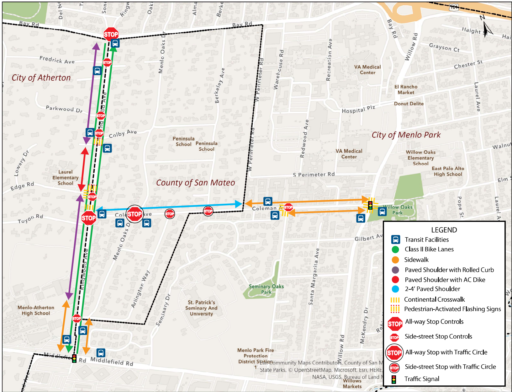
Coleman and Ringwood Avenues Transportation Study - Existing Conditions Figure 3 – Intersection Controls and Existing Pedestrian, Bicycle, and Transit Facilities
